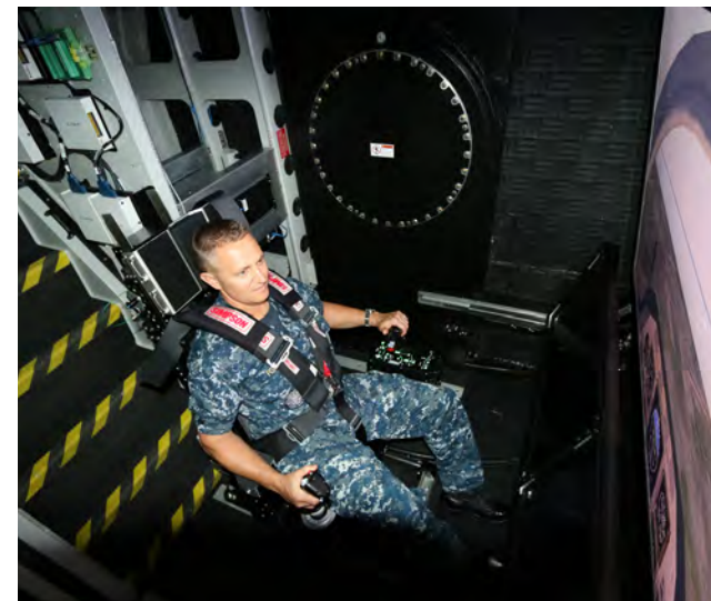
The author is strapped in prior to a test of a man-in-the-loop mode where subjects can control the device from inside the capsule. Photo by Megan Mundersbach
